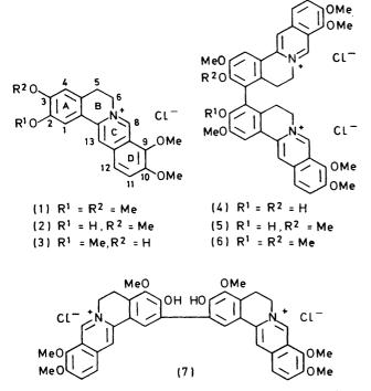
In order to confirm this suggestion, methylation of the phenolic groups with dimethyl sulphate  $^{12,13}$  was attempted. After isolation *via* column chromatography we obtained a fully methylated compound (6) and only one monophenolic compound (5). The u.v. and visible spectra of these compounds confirmed their protoberberine character. In the n.m.r. spectra, the aromatic region and (particularly) the number of methoxy-groups provided strong evidence of a dimeric structure.
